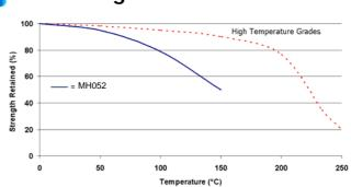
The reduction in strength shown here is reversed on cooling providing the joint is not overstressed. Exposure to higher temperatures may be acceptable for short periods
